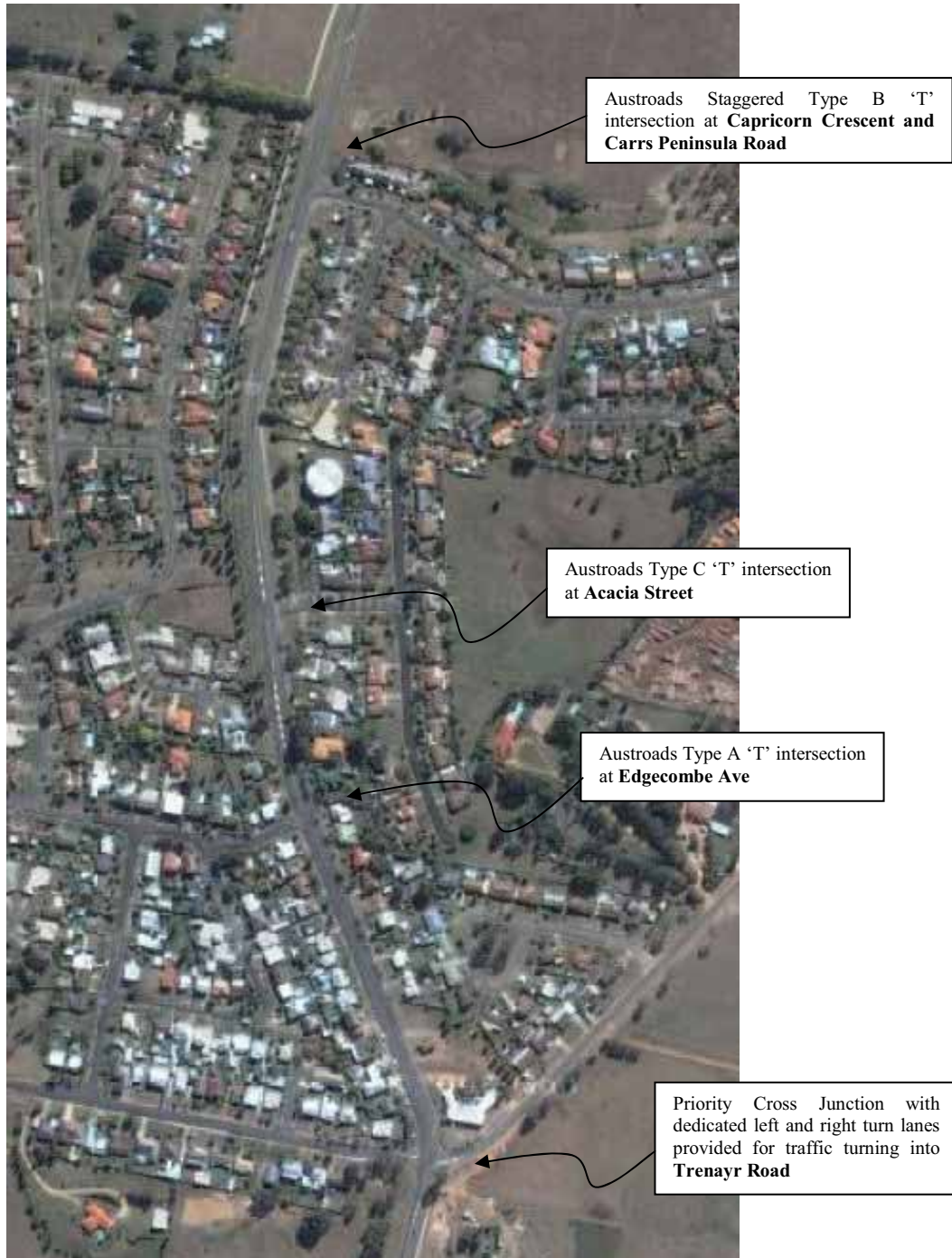
FIGURE 3.1 – EXISTING INTERSECTION CONDITIONS ON THE SUMMERLAND WAY THROUGH JUNCTION HILL
